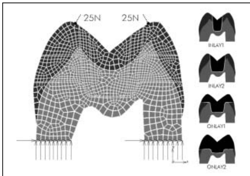
**Fig 1** Original natural contours and mesh developed in MENTAT (left). The two 25-N occlusal loads are applied to cusp tips, just within occlusal table (dotted lines = load direction). Horizontal and vertical fixed displacements are shown at cut plane of root (arrows). Four restorative designs (right) were reproduced using same original mesh.
